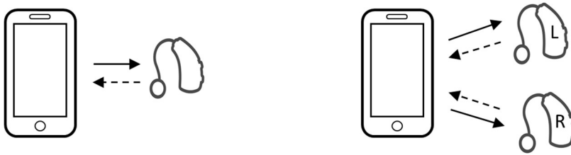
Figure 2.1 Basic Hearing Aid topologies
