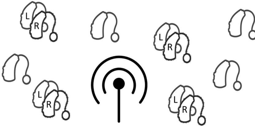
Figure 2.4 A broadcast topology to replace telecoil infrastructure
