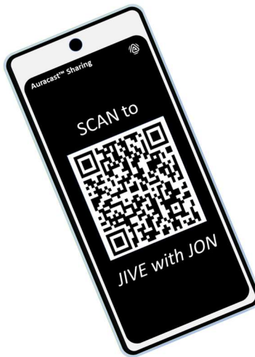
Figure 11.13 An example of a QR code generated to allow sharing of audio content from a smartphone.
